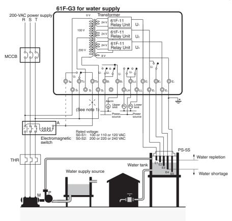
Note: 1. The diagram shows the connections for the water supply. When draining, change the connection from terminal Tb to terminal Ta.
