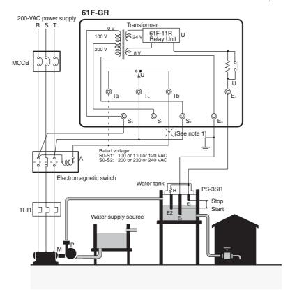
Note: 1. The diagram shows the connections for the water supply. When draining, change the connection from terminal Tb to terminal Ta.
