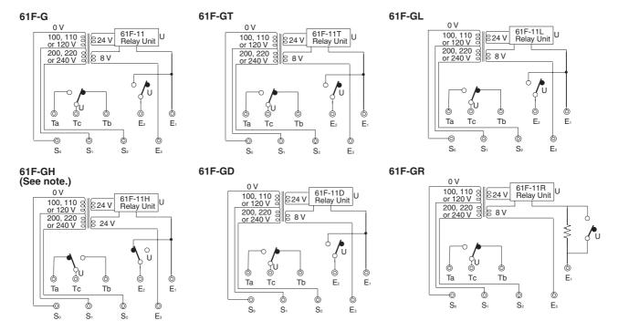
Note: The 61F11H relay deenergizes when there is water present across the Electrodes, whereas the 61F relay energizes when there is water present across the Electrodes.
