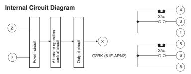
Connect the output terminal Ta of the 61FG□ to input terminal 2 of the 61F-APN2.
