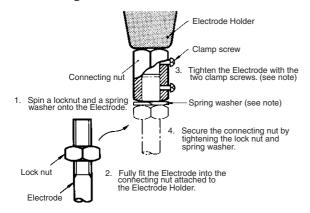
Note: Clamp screw and spring washer are not provided for the BS-1T Electrode Holder (titanium, hastelloy B, or hastelloy C).
