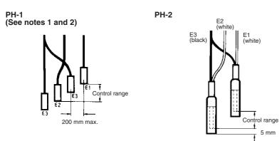
Note: 1. When the distance between E1 and E3 exceeds 1 m for supplying purified city water, for example, locate a second E3 within 200 mm of E1
