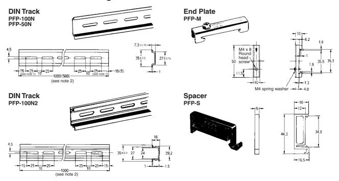
Note: 1. The PFP-100N is 15 mm on both ends, while the PFP50N is 15 mm on one end and 5 mm on the other end.
