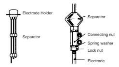
When the required length of Electrode is more than 1 m, use a Separator at each joint of two Electrodes so as to prevent the Electrodes from contacting one another.
