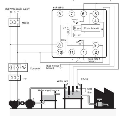
Note: 1. The diagram shows the connections for the water supply. When draining, change the connection from terminal 1 to terminal 11.
